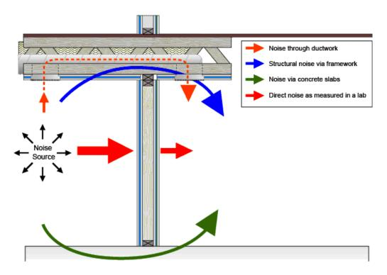
The red arrows in the sketch above are direct noise, noise passing through the wall into the next room. The orange, blue, and green arrows reflect noise that can make it into the next room via paths not related to the wall. Noise coming from these paths is called "flanking noise."
