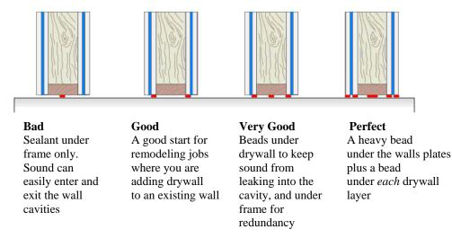
You should strive for multiple caulk layers on partitions where sound isolation is critical. This helps ensure that a quality seal is attained by "doubling up" on seals - if one layer has compromised quality, it is backed up by the other layers.
