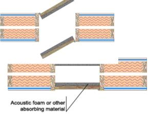
doors. It is completely reasonable to consider two heavy communicating doors preferable to any realistic single door, engineered or not. If you opt for communicating doors, it is a great idea to put some type of sound absorption in the cavity between the two doors. Cloth-wrapped rigid fiberglass or acoustic foam are two excellent choices.
