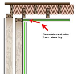
Structure-borne noise is reduced, as there is no mechanical path from noise to the main structure of the construction.
