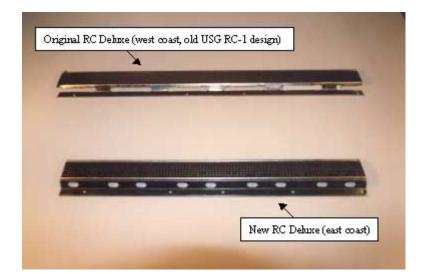
A little-known (but important) design element of the original USG resilient channel is the location of the framing member in relation to the slotted holes. If you look at the original RC-1 design you will note that there are 1/8" diameter holes every 4 inches for screws to attach the channel to the framing members.
